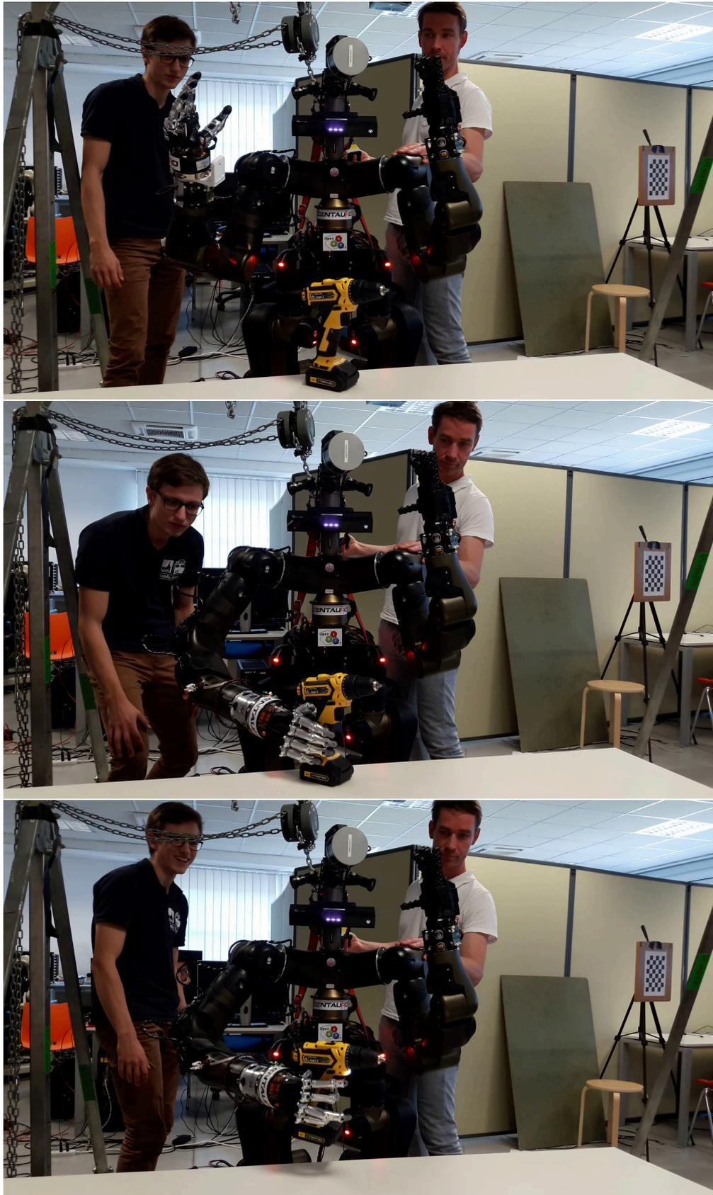
Figure 7.33: Centauro robot grasping novel drill using the results of the pipeline proposed in this thesis.
