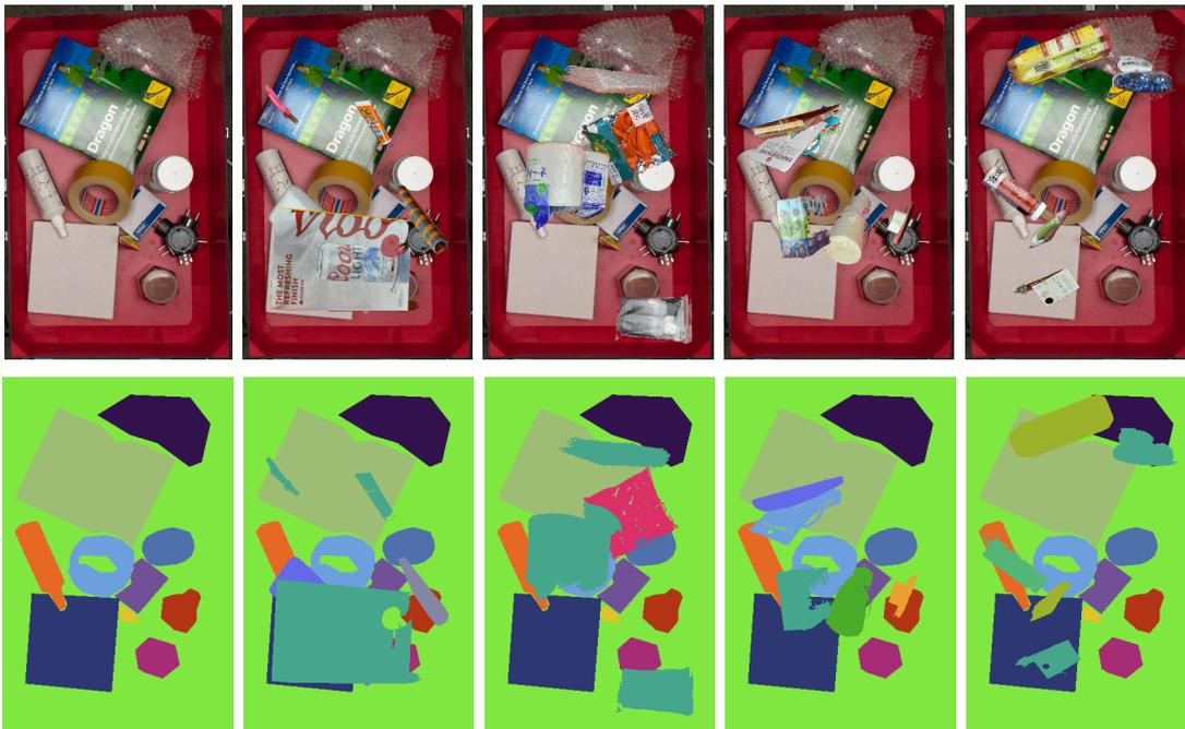
Figure 3.4: Generated synthetic scenes. All scenes were generated with the same annotated background frame (left column) for easier comparison. Top row: RGB. Bottom row: Color-coded generated segmentation ground truth. Source: Schwarz, Lenz, et al. (2018)
