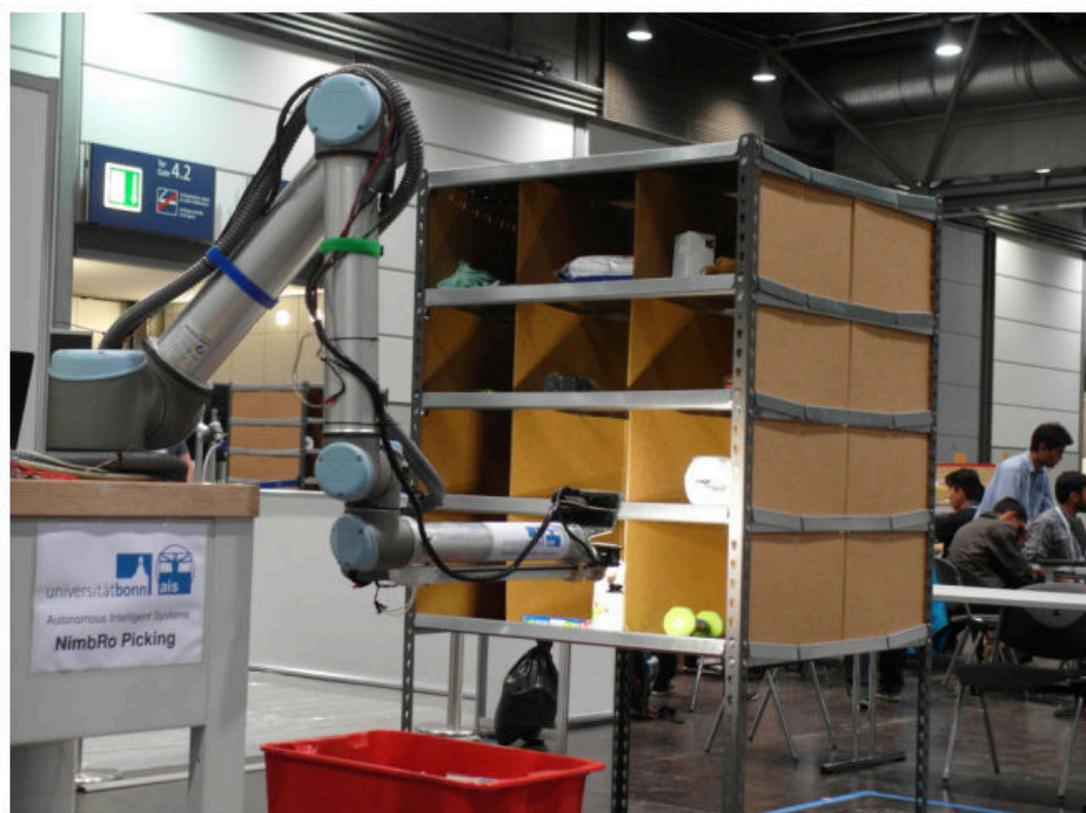
Figure 2.2: Team NimbRo's robot picking objects from the shelf and placing them in the red tote. Source: Schwarz, Milan, et al. (2017).
