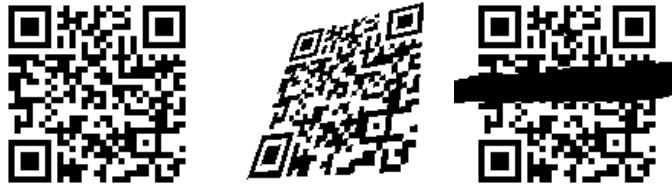
(a) readable QR image. (b) an distorted image. (c) blobby or blocked image.
