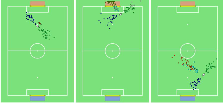
**Fig. 3.** Three examples for kick simulations. Each possible kick direction is simulated with 30 samples (different colors correspond to different kicks). Left: the short and long kicks are shortened due to collision with an obstacle. Middle: long kick is selected as the best action since it has the most samples result in a goal. Right: the best action is sidekick to the right – the other kicks are more likely to end up in a dangerous position for the own goal according to the potential field.
