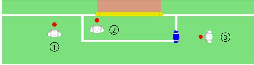
**Fig. 1.** Depictions of three different situations in which the best decision is not clear. The white robot is the robot having to take a decision on which (kick) action to perform while the blue robot is an opponent. The ball is depicted in red.
