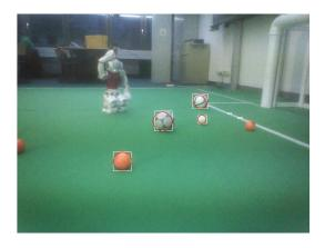
Figure III.1. The result of the ball detection as seen in the HULKs debug tool. Clustered regions are highlighted white, detected balls are circled red. Note, that the 2016 ball candidate is detected.
