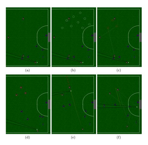
**Fig. 7.** a) Initial setup for servicing a free kick for the STOx's team. b) Locations found by the described algorithm are shown in white circles on the field. c) Three selected locations shown in red circles to send the three available attackers. d) The three attackers has been placed in to the three selected locations. e) The pass is made to the attacker with higher scoring chance. f) The attacker receives the pass and shoots at goal, finally scoring.
