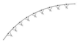
Fig. 3. Angles between ten consecutive apparent ball positions in a parabolic shot
