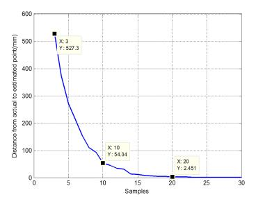
Fig. 5. Average error of the estimated final point for all 60 kicks for a different number of samples used to reconstruct the parabolic paths.
