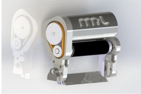
Fig. 21. New dribbling system of the MRL robot
