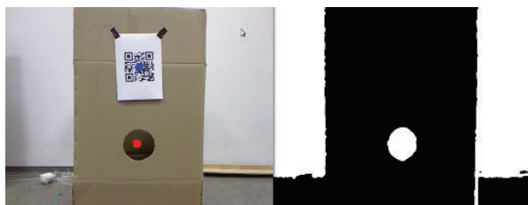
Fig. 5. The results of the developed system (left) QR-code is marked by blue dot while the hole is pointed out by red one and (right) black/white image obtained by medianization in the first step of hole detection.
