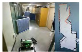
Fig. 8. Photo of SLAM test
