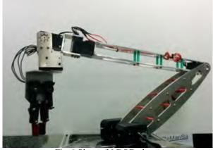
Fig. 6. Photo of 6-DOF robot arm
