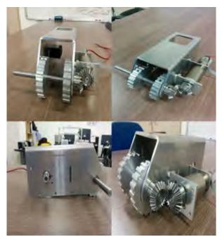
Fig. 3. Photo of robot's main driving part (one module)
