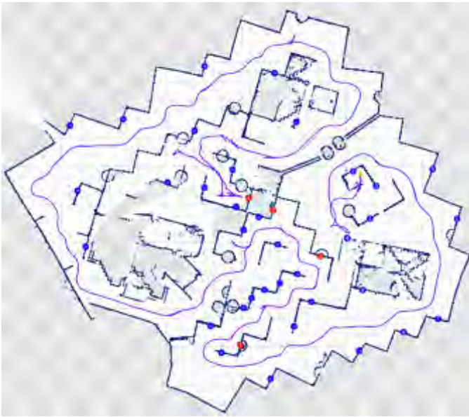
Fig. 3: Map learned using the hector_slam system at the final mission of RoboCup 2012. The robot started at the right middle position and autonomously explored the majority of the arena, finding 3 victims (red markers). The fourth victim was found using tele-operation on the last 4 meters of the travelled path. Blue markers indicate the positions of 35 QR codes that were detected autonomously by the robot.
