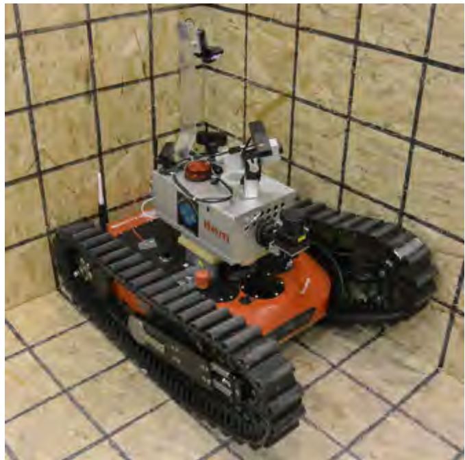
Fig. 1: The Taurob Tracker platform as adjusted for autonomous use at the RoboCup 2015 competition. For the 2016 competition, an arm will be mounted on the robot and full 3D LIDAR capability will be added using a sensor mounted on a slip ring.
