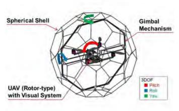
Fig. 1. The PRSS UAV can be devided into three parts; an internal UAV, a 3-DoF gimbal, and a shell. The structure of the shell is so-called fullerene, which gave us an idea of the team name. An introduction video of the PRSS UAV is available at https://youtu.be/c1fMsK-qBX4
