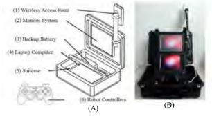
Fig. 9. BART LAB Rescue Robotics operator station: (A) CAD design (B) Our Operator's Station
