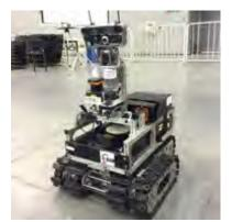
**Fig. 2.** Autonomous robot of BART LAB Rescue Robotics team, AutoBot IV. This robot has a track-based locomotion system with sensors for the victim identification system, which uses image processing and heat imaging technology.
