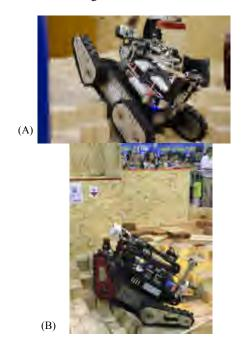
Fig. 1. TeleOp IV - our previous version (A) and TeleOpV (B) are the two tele-operative robots in BART LAB Rescue Robotics Team. Both robots employ track locomotion with four independent flippers, and are equipped with manipulator which is controlled using inverse-kinematic algorithm for their capabilities in search and retrieve victim information, similarly to robots in [1, 2].
