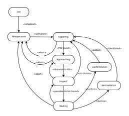
Fig. 2. State machine for autonomous behaviour.
