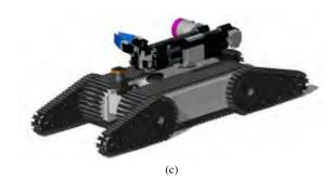
Fig. 1. Robot's of team AutonOHM: Georg (a) is used for autonomous driving and exploration. Robot Simon (b) can further be used for teleoperated driving. The new robot (c) will be capable of driving in rough terrain. Equipped with a manipulator it can inspect points of interest up to a height of 1.5 meters.
