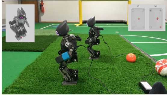
Fig. 1. Robots actively maintaining stability. Robot 2 (right) is equipped with FSR foot sensors and controls measured COP to be in the centre of support polygon. Robot 5 (left) has no foot sensors but derives stability reference point from IMU and orientation and controls this reference point to be within support polygon
