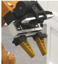
Fig. 2: Custom designed gripper for grasping a wider range of objects.
