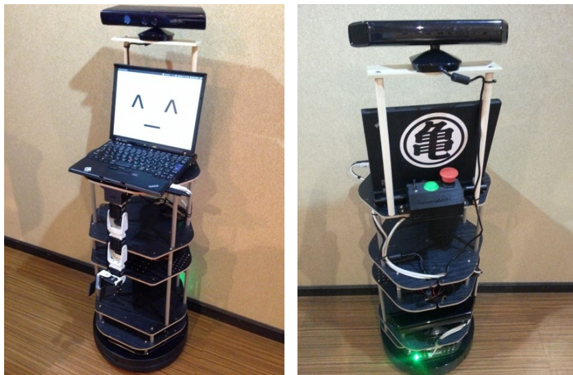
Fig. 1. The first working prototype of the open robot platform for RoboCup @Home
