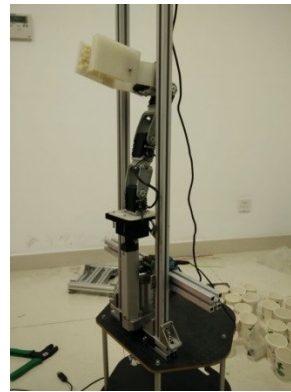
Fig. 5. Elevated arm for flexible height manipulation
