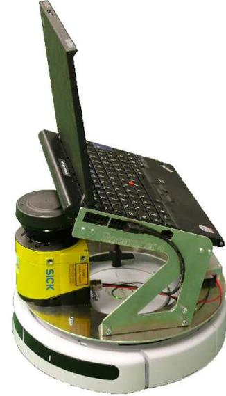
Fig. 2. RoomRider: the teaching and research platform from the Autonomous Intelligent Systems research group of the University of Bonn, with a Roomba vacuum cleaning robot as basis, a SICK S300 laser range sensor and the controlling notebook on top, photo by courtesy of M.Schreiber.
