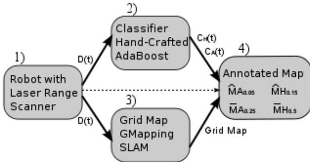
Fig. 1. The approach is structured into 4 major functional blocks:  $\mathbf{D}(t)$  distance measurement,  $\mathbf{C}_H(t), \mathbf{C}_A(t)$  class membership vectors, annotated maps  $\hat{\mathbf{M}}_{H_Z}, \hat{\mathbf{M}}_{A_Z}$ , created with the different methods  $\hat{1}$  and  $\hat{2}$ , and with different spatial resolutions  $Z$ .
