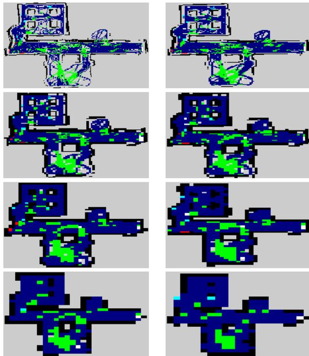
Fig. 7. Semantic map of `World10` created with the hand-crafted classifiers using method 1 for the annotation  $\hat{\mathbf{M}}H_Z$  with  $Z$  the respective cells sizes from top left  $Z = 0.05m$  to bottom right  $Z = 0.5m$ , 0.05,0.10, 0.15,0.20, 0.25,0.30, 0.40,0.50.
