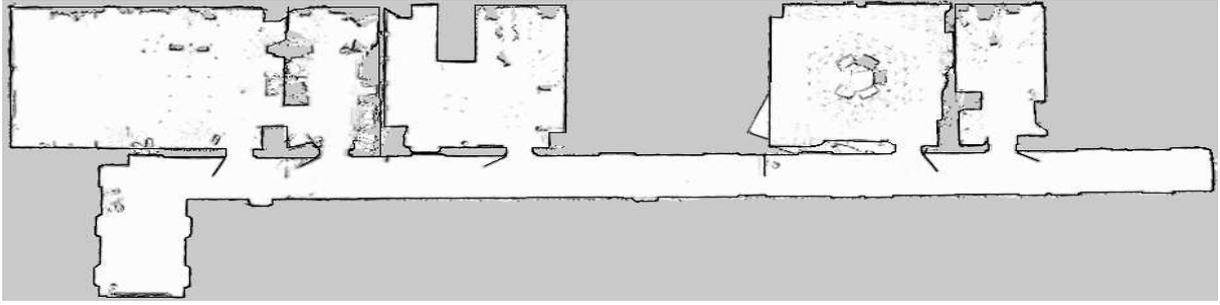
Fig. 5. `World9`, map created with GMapping, containing doorways, a corridor, freespace regions and several rooms, the door leafs are clearly visible, and have not been erased from the map, the cell size is  $0.05m$ . The map has been reworked manually with a drawing program to get a closed contour for the walls which is necessary for the simulations.
