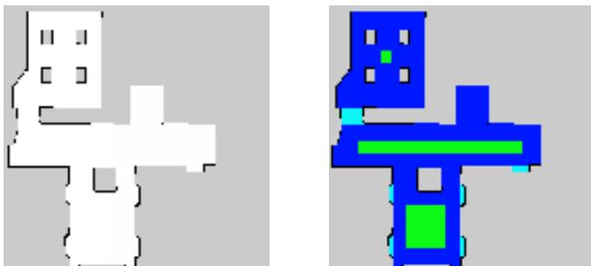
Fig. 3. World10: left: result from GMapping; right: grid map annotated with human generated "ground truth" data.
