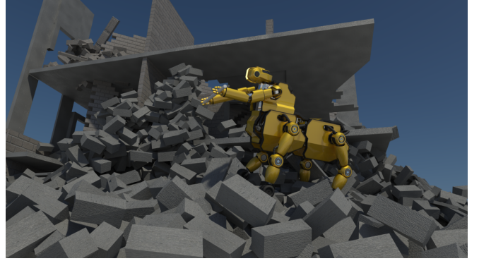
Fig. 1: Basic idea of the CENTAURO project – the joint hardware/software development of a teleoperated robotic field system for disaster-response.
