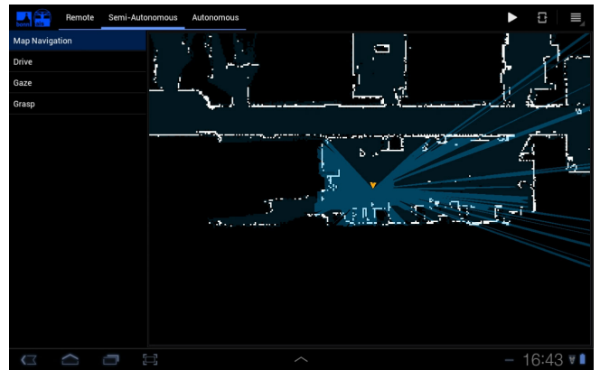
Fig. 5. Skill-level teleoperation user interface for navigation in a map. It visualizes the location of the robot and overlays the current measurements of the navigation laser sensor. The user can specify the navigation goal pose by touching onto the goal position and dragging towards the desired robot orientation at the goal.
