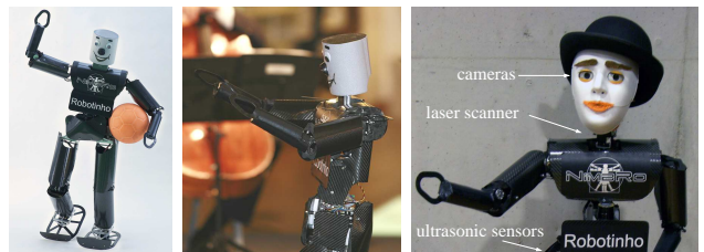
Fig. 2. Our robot Robotinho was initially used as soccer player in the RoboCup Humanoid League. He conducted The 12 Cellists of the Berlin Philharmonic in September, 2006. The right image shows the communication head as well as the position of the cameras and distance sensors.
