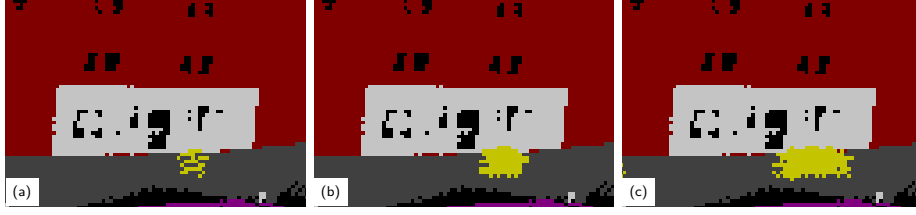
Figure 5: Paris-CARLA-3D dataset: Projection of dynamic persons (yellow) into the virtual OS0 LiDAR view using dataset scans from (a) only the current, (b) \pm 2 , and (c) \pm 5 adjacent positions. The foreground person is incomplete when using just a single scan (a) but significant movement artifacts appear for a larger scan window (c). We use a window of \pm 2 (b) for our experiments as compromise between complete scans and remaining artifacts.
