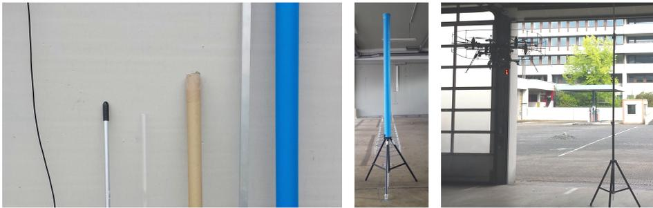
(a) Left: Different object types, from left to right: cable (∅0.75 cm), aluminium broomstick (∅2.7 cm), plexiglass tube (∅5 cm), cardboard tube (∅7.5 cm), rectangular metal rod (∅4 cm), blue plastic tube (∅11 cm). Middle and right: experiment setup with object holder, measuring tape and flying multicopter.
