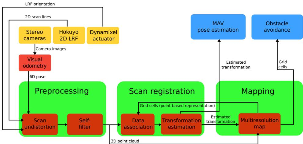
**Fig. 3:** An architectural overview of our system. The LRF measurements are processed in preprocessing steps described in Section 4. The resulting 3D point cloud is used to estimate the transformation between the current scan and the map as described in Section 5. Registered scans are stored in a local multiresolution map.
