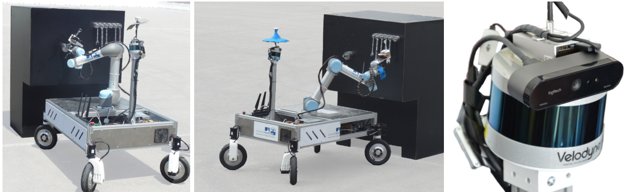
Figure 1: Left: Mario turning the valve during practice. Center: Mario grasping the correct wrench during the Challenge 2 finals. Right: Mario’s sensor head with 3D laser scanner, DJI Flight Controller, and webcam.
