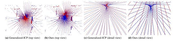
**Figure 2:** Registering two point clouds (red and blue points) in an example scenario: the original Generalized-ICP implementation suffers from the degradation of the underlying covariance matrices and incorrectly aligns the two point cloud origins and the individual scan lines (a,c). Our approach correctly registers the two point clouds (b,d).
