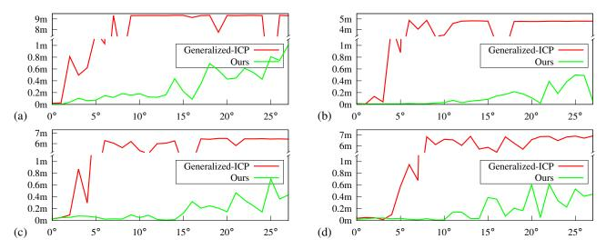
**Figure 3:** Evaluation of the divergence behavior on four scan pairs (a-d). Registration (translation) errors increase with an increasing angle  $\theta$  between scan lines. Our approach can compensate for non-uniform densities and achieves fairly acceptable results even for larger angles between scans.
