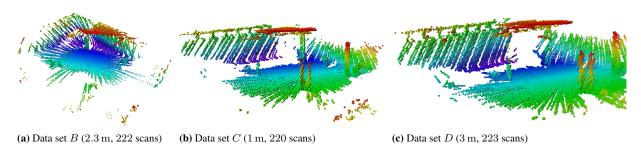
**Figure 6:** Visualizations of the (local) 3D maps built from the other selected data sets. All data sets are available at: http://www.ais.uni-bonn.de/may registration.
