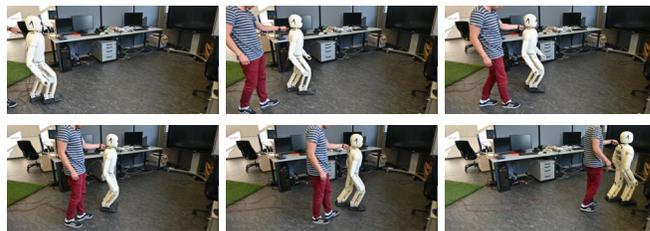
Fig. 5. Snapshots of forward walk performed by the real robot commanded by the learned locomotion controller.
