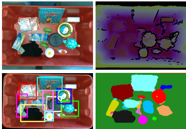
Fig. 4. Object perception example. Upper row: Input RGB and HHA depth frames. Lower row: Object detection and semantic segmentation results (colors are not correlated).
