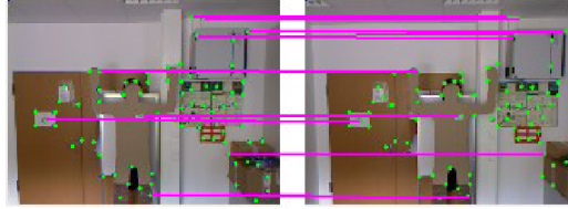
Fig. 2. Features in one frame (previous) are tracked during the tracking process to the next frame (tracked features TF ). Some of the correspondences are shown in magenta.
