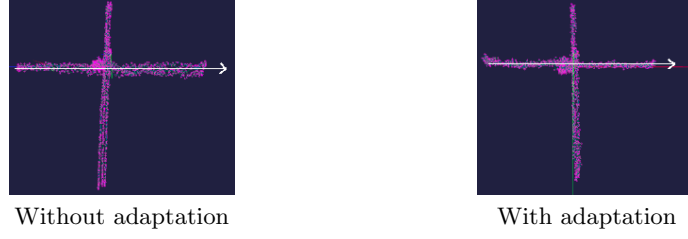
Fig. 6. Effect in the adaptation of the consistency. The distance from the sensor to the features increases in the direction of the arrow. Notice that the dispersion of the position increases with the distance to the sensor when no adaptative consistency is used
