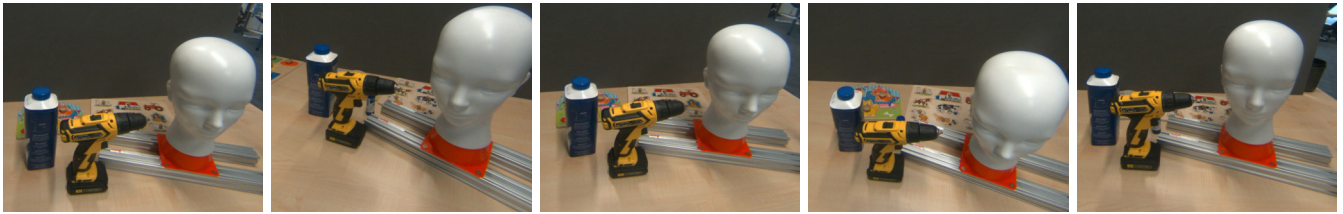
Fig. 2. Range of motion supported by our setup. We show the left eye view of the HMD, cropped to the central part for clarity. Note that the human operator can easily change perspective and observe parts of the scene that were previously hidden.
