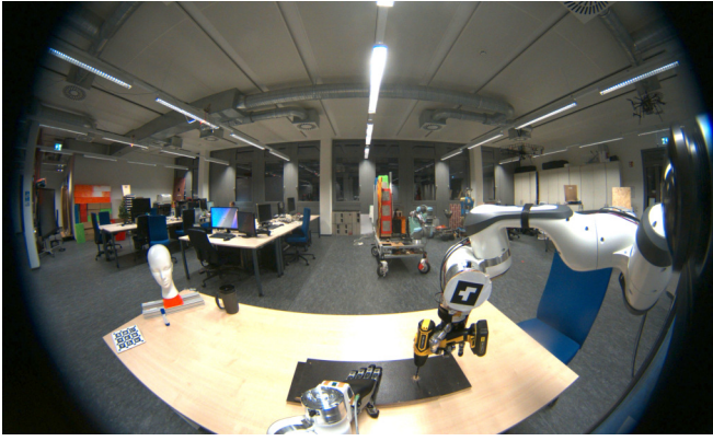
Fig. 3. Raw image from one of the wide-angle cameras. The horizontal field of view is higher than 180°.
