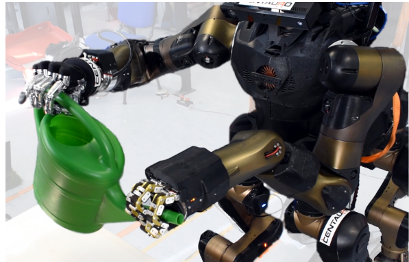
Fig. 1. The Centauro robot performing bimanual grasping of a novel watering can.
