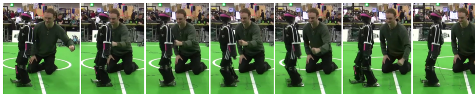
Fig. 1. Humanoid robot Dynaped regaining balance by stepping forward after a push from the back.
