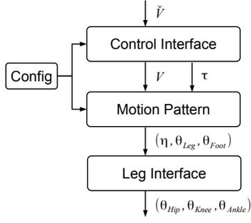
Fig. 2. Hierarchical layers of the Nimbro gait generator. The Control Interface receives a gait velocity target  $\check{V}$  from a higher layer and translates it to a bounded and smoothed gait velocity vector  $V$ . The Motion Pattern layer generates phase  $\tau$  dependent periodic motion signals on an abstract level that is translated by the Leg Interface to joint targets.
