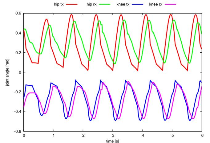
Fig. 5. Time series of the commanded (tx) positions and measured (rx) positions of the right hip pitch and knee joints during forward walking.
