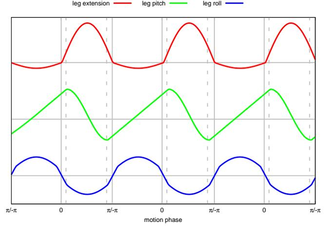
Fig. 4. The main ingredients of the gait motion are rhythmic leg lifting (top), leg swing motion (center), and a lateral hip swing (bottom). Only the patterns for the right leg are shown. The solid vertical lines indicate the expected times of support exchange. The dashed vertical lines indicate the swing start and swing end timings.
