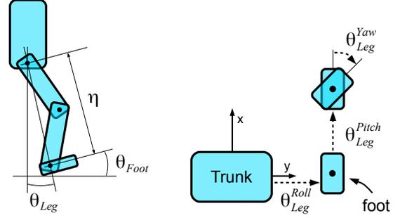
Fig. 3. The Leg Interface allows independent control of three abstract parameters: the leg extension  $\eta$ , the leg angle  $\theta_{Leg}$ , and the foot angle  $\theta_{Foot}$  (left). The leg can be bent independently in roll, pitch, and yaw directions (right).
