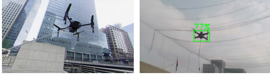
a) Synthetic DJI M100 drone b) Detection in real image Figure 7: Synthetic data can be easily rendered and used for deep learning applications. Images of drones together with ground truth bounding box annotation were rendered and used for training a drone detector.
