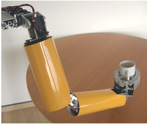
Fig. 3. 7 DOF human-scale anthropomorphic arm with 2 DOF gripper.
