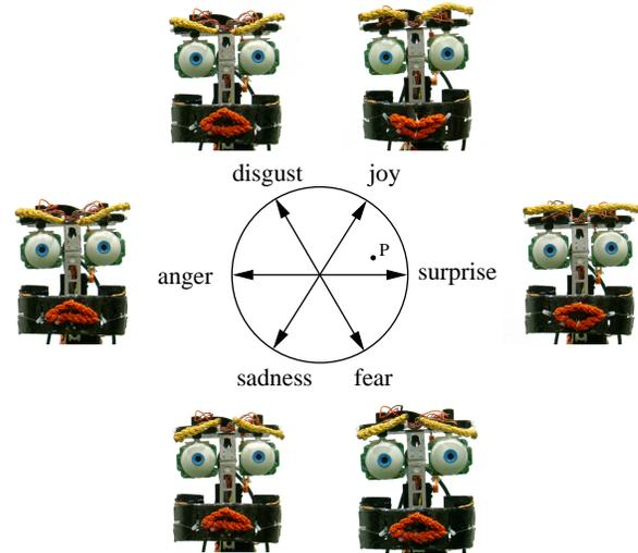
Figure 6. The two-dimensional space in which we compute the robot's mood. The images show the six basic facial expressions of our robot. The mood corresponding to a point  $P$  is computed according to Eq. (1).
