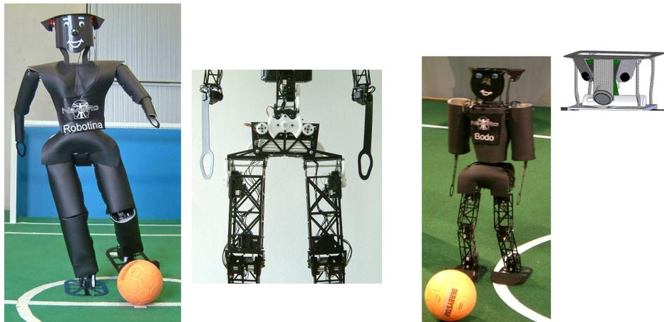
**Fig. 2.** NimbRo TeenSize 2007 robots Robotina (left, with mechanical detail) and Bodo (right, with drawing of new camera head)
