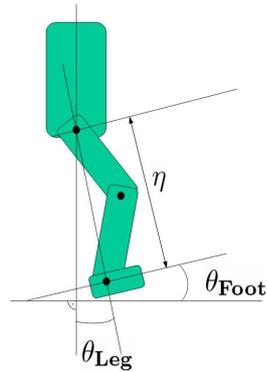
**Fig. 4.** Kinematic interface to a leg.
