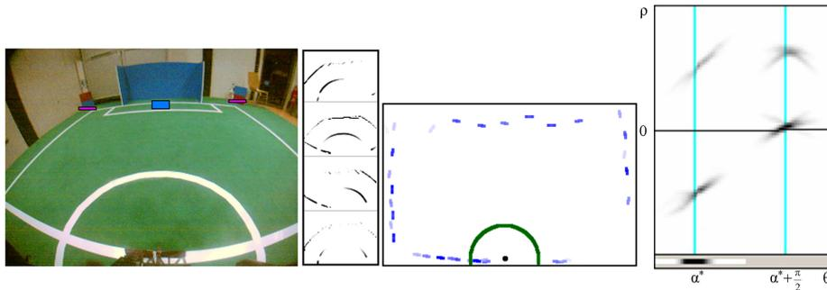
**Fig. 3.** Detection of field lines (left to right): image captured by a walking robot, responses of four orientated line detectors, oriented line segments with removed center circle, Hough space with major orientation  $\alpha^*$  and main lines.
