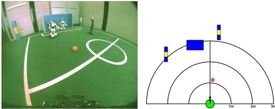
**Fig. 2.** Left: View onto the soccer field captured from the ultra-wide-angle FlyCam. Right: Egocentric coordinates of key objects (ball, goal, corner poles) detected in the image.
