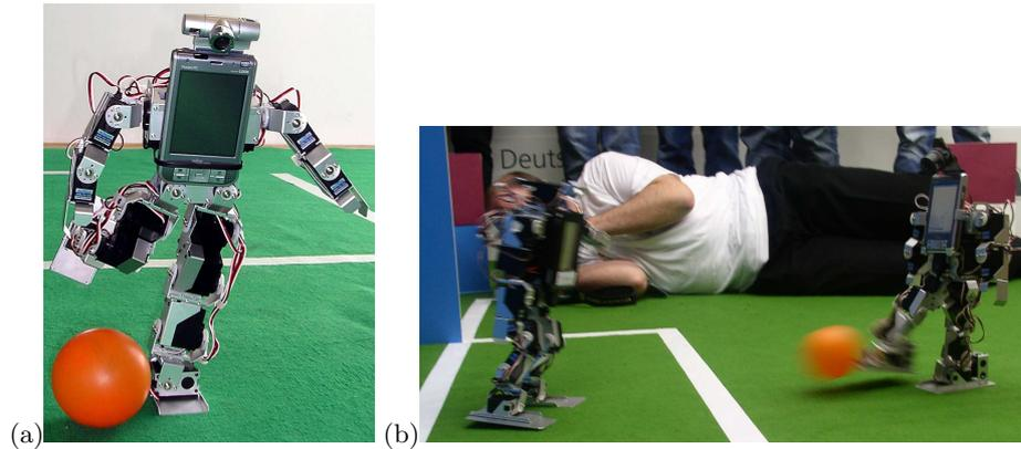
**Fig. 2.** (a) Augmented Kondo robot. (b) Penalty Kick demonstrations at German Open 2005: Darmstadt Dribblers vs. NimbRo.
