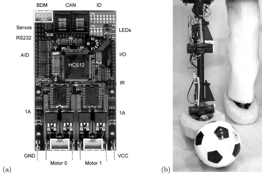
**Fig. 2.** (a) HCS12 electronics board; (b) two legs (one exposed, one covered with soft material) consisting of a 3DOF arm and a 2DOF foot each, attached to the lower part of the trunk.
