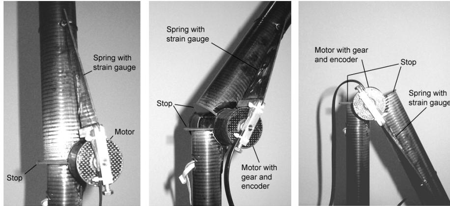
**Fig. 1.** Knee joint, constructed from carbon composite tubes and sheets. The DC-motor and the flat spring form a series elastic actuator [6]. The strain gauge measures the bending of the spring, which is proportional to the actuator torque.
