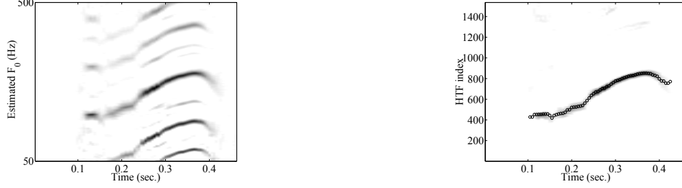
Fig. 2. (a) Harmonic template function for pitch estimation using 2 to 10-pitch period windows of length 400 to 800 for the utterance “The north” (male). (b) Final HTF after applying feature extraction operations. The circles show the path found by the pitch tracking algorithm.
