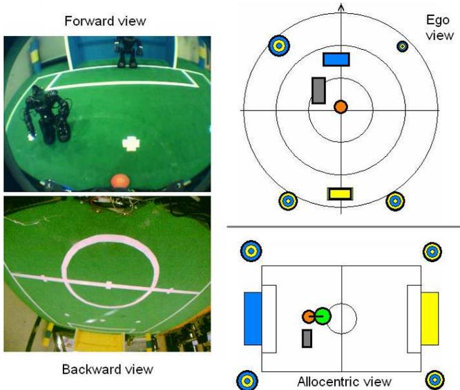
Fig. 3. Left: Images of the two cameras mounted on a KidSize robot. Upper right: Egocentric coordinates of key objects (ball, goals, corner poles, obstacle) detected in the image. Lower right: Localization of the robot, the ball, and the obstacle on the soccer field.
