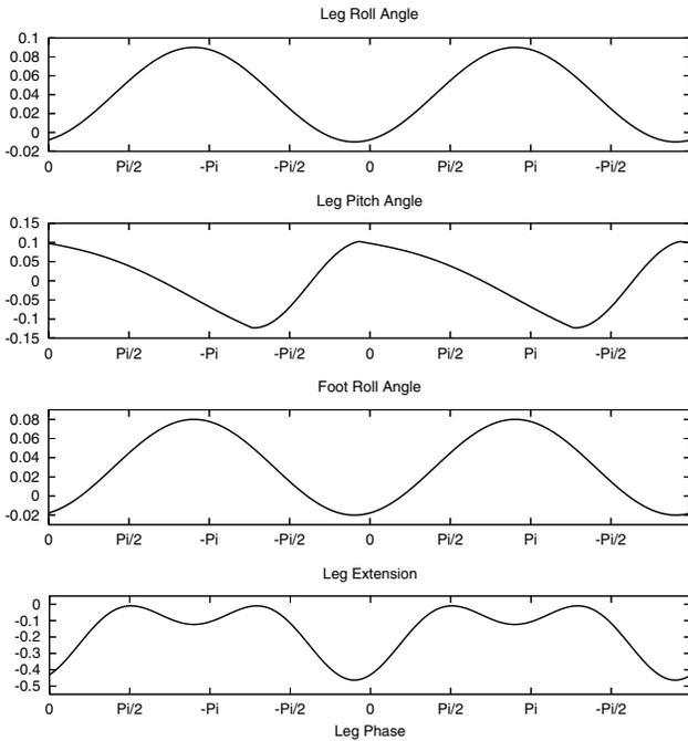
Fig. 6. Trajectories for forward walking of KidSize robot.
