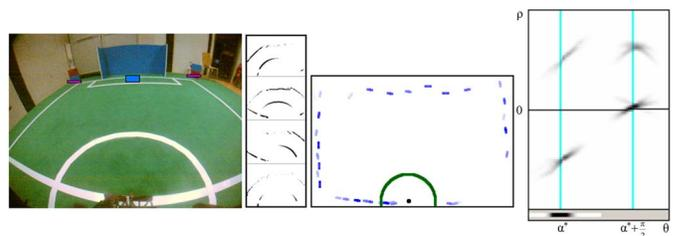
Fig. 4. Detection of field lines (left to right): image captured by a walking robot, responses of four orientated line detectors, oriented line segments with removed center circle, Hough space with major orientation  $\alpha^*$  and main lines.
