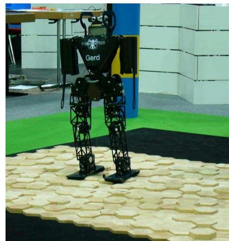
Fig. 10. RoboCup 2006: KidSize robot Gerd walking over rough terrain.
