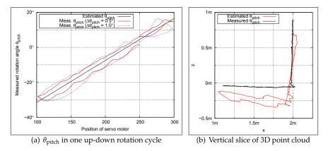
Fig. 12. Estimated and measured pitch angles. Depending on the gear backlash, pitch angles estimated based on the position of the servo motor may deviate from the actual pitch angle (a). Measuring the pitch angle, e.g., using gyroscopes still yields accurate and correct geometric information (b).
