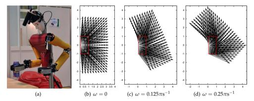
Fig. 17. The anthropomorphic service robot Dynamaid (a) and look at points **g** for different configurations of  $\mathbf{v}^x$ ,  $\mathbf{v}^y$  and  $\omega$ .
