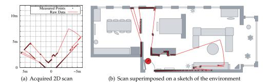
Fig. 1. 2D laser range scan in an example scenario. Depicted is a range scan (a) from a data set recorded by Zivkovic et al. (2007) together with an approximate floor plan of the scenario (b). Note, that the couch table has not been sensed at all since it did not intersect the scanner's measurement plane.
