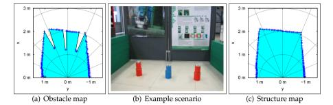
Fig. 6. Demonstration of the virtual 2D map types in an example scenario. The *obstacle map* (a) is generated by extracting minimum distances (projected into 2D) in the continuously acquired 3D data. Extracting maximum distances results in the *structure map* (c).
