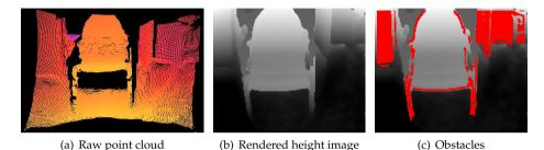
Fig. 13. Detecting obstacles in range images. Based on the acquired range image (a), a height image (b) is constructed. Filtering the height image results in the set of obstacle points (c).
