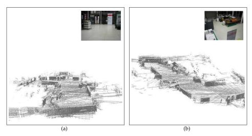
Fig. 11. Different views on the complete 3D model. It can be seen that the map does only model environmental structures in a height of the robot. That is, only those regions are modeled with which the robot can interact.
