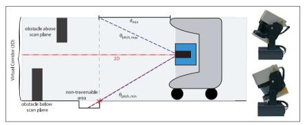
Fig. 4. Continuously pitching scanner and virtual corridor. By continuously rotating the scanner in a nodding-like fashion over the area of interest (AOI), all obstacles in the virtual corridor are perceived.
