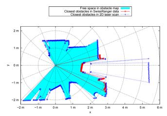
Fig. 15. The resulting *virtual scan* of the scene is compared with the base laser scan. The base laser scan is illustrated by the dashed green line. The red line illustrates the virtual laser scan. The chair shows only a few points in the base laser scan since only the legs of the chair are in the scan plane, whereas the *virtual scan* outlines the contour of the chair.
