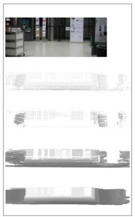
Fig. 9. Example of a generated point cloud. The figure shows (from top to bottom): a photo of the captured scene, the range measurements acquired during movement, the reduced set of points (without floor points), detected lines and a rendered depth image.
