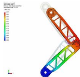
Fig. 3. Example of FEM simulation to validate the stiffness of the legs.
