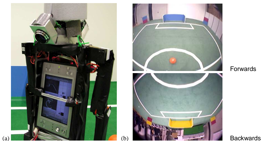
Figure 1: Toni with a small PC and two ultra-wide-angle cameras: (a) Picture of the robot's back and neck; (b) Pictures captured simultaneously from the two cameras.
