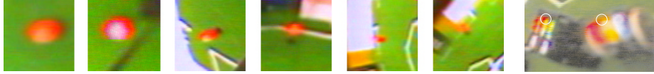
Fig. 3. The ball's appearance varies in color and shape and is similar to robot markers.
