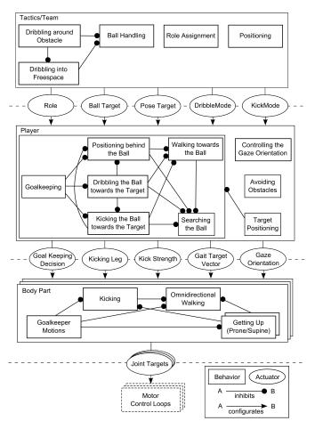
Fig. 5. Actuators, behaviors, and mutual inhibitions within the behavioral hierarchy. Upper layer behaviors can configure lower layer behaviors by manipulating the upper layer actuators. The resulting values of the actuators depend on the activation factors and the inhibitory structure of the manipulating behaviors.
