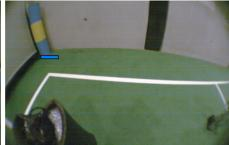
Fig. 3. Images captured by the three cameras. The detected objects are marked: goals (blue and yellow rectangle), ball (orange circle), field makers (gray circles), corner poles (horizontal blue and yellow lines), goal post (white circle), and obstacles (white vertical rectangles). The free goal area is marked on the left and the right of the goalie with a green and red line, respectively.
