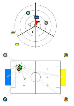
Fig. 4. Egocentric and allocentric representations of the game situation constructed by the computer vision module.
