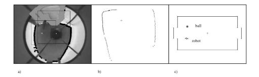
**Fig. 1.** Detection of ball, goal and localization of the robot: a) Transition search, ball and goal detection; Black dots correspond to found transitions between the wall and the field. Rectangles (their centers) mark the ball and the goal. b)Obtained range scan after transforming the points; c)Localization of the robot in global coordinates;
