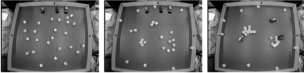
Figure 3.3: Example of heap building by Didabots. Initially the cubes are randomly distributed. Over time, a number of clusters start to form. In the end, there are only two clusters and a number of cubes along the walls of the arena.
