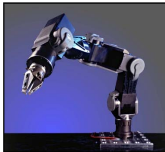
Torque sensors after the gears, but before the last bearings
