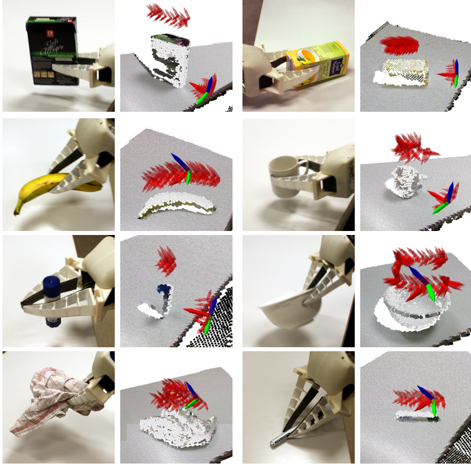
Figure 9: Example grasps and grasp planning results for each of the eight household objects used in the experiments. For each object, we visualize the best grasp that is executed (larger RGB axes) and sampled grasps (smaller red axes) by their pre-grasp pose.
