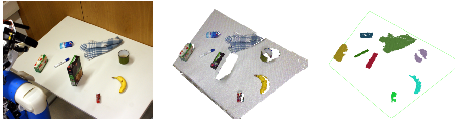
Fig. 2. Object detection. Left: example table top setting. Center: raw point cloud from the Kinect with RGB information. Right: each detected object is marked with a distinct color.
